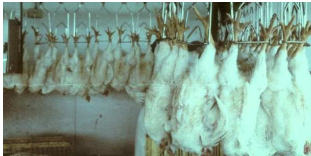
Birds hung consciously by both legs on a shackle line before going through a waterbath for stunning.
